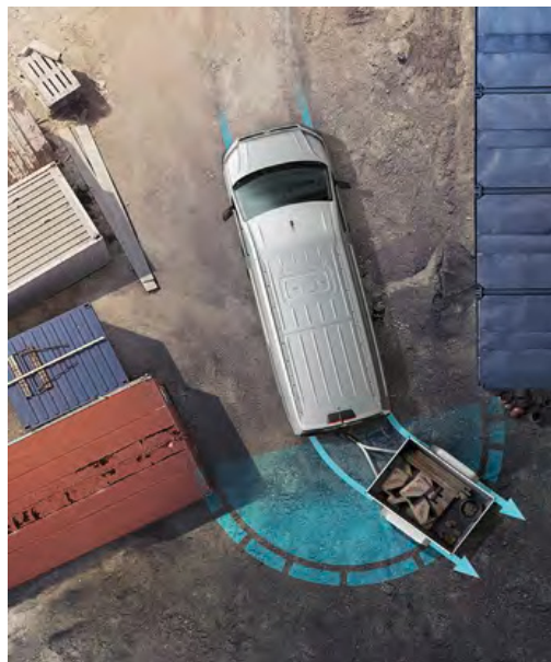
Trailer maneuvering assistant "Trailer Assist" (Schematic representation using the example of the Crafter model).
